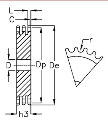
C = 1 D = 25 De = 247.1 Dp = 242.61 For chain size =  $3/8 \times 7/32$ For chain type = 06 B-3 h3 = 25.6 L = 5.2 Number of teeth = 80r = 6.35
